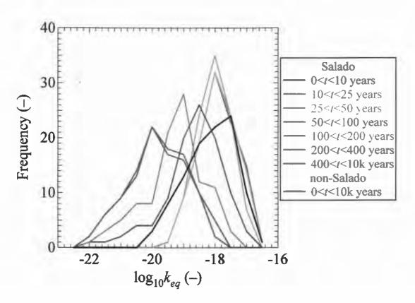
Figure 3: Distribution of equivalent permeabilities for the PAVT R1 shaft. Note that change in color represents the distribution of equivalent permeabilities over a different time interval.
