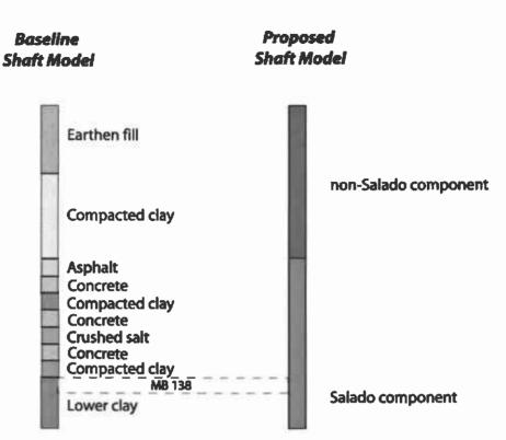
Figure 2: Representation of the baseline shaft seal model contrasted with the proposed simplified model.
